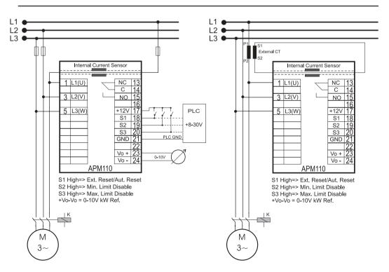
Fig.4 Typical connection with internal sensor
