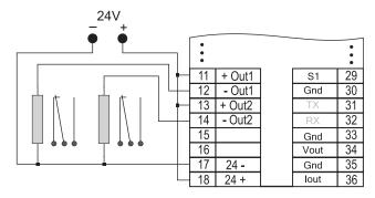
Figure 3 Ex. with digital outputs connected to external relays
