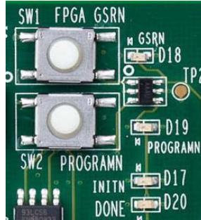
Figure 3. LatticeECP3 Status LEDs and Push-button Controls
