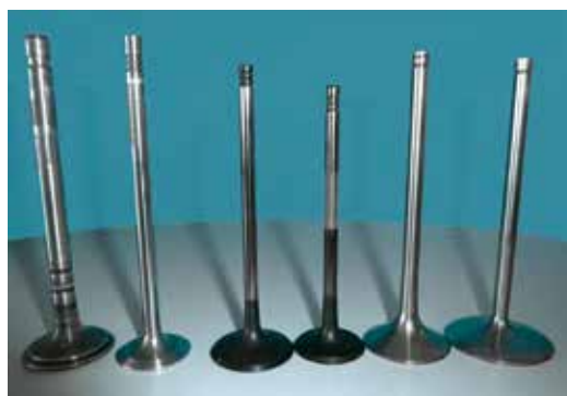
Fig. 4: Inlet valves with tooth structure on valve stem
