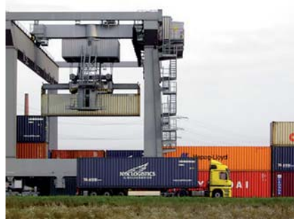
Suspended loads can be positioned accurately thanks to motor and encoder feedback.
