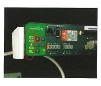
2. Press key "M" 2 times, HMI display P0-00
