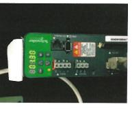
3. Press "ok", HMI display 01.30, means the first 4 figures of FW sion
