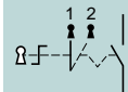
Selector switch 2-position stay put, key withdrawal from both positions N/O contact
