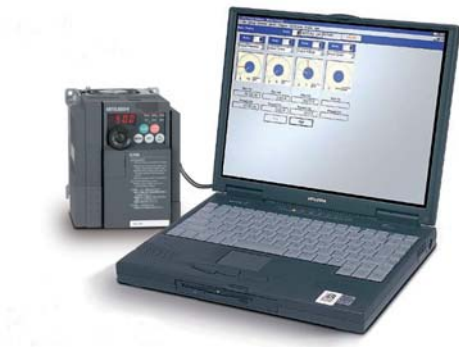
Configuring the drive via a Windows laptop
