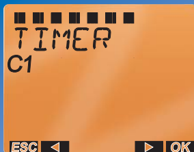
Countdown timer Time can be set between 1 min. and 23 hrs. 59 min.
