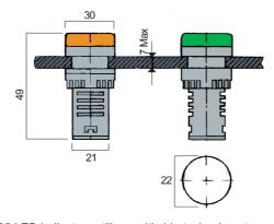
IP65 LED indicators utilise multi-chip technology to provide bright even colour in red, blue, yellow, white and green. An aesthetically appealing design featuring single back of panel lock-nut fixing and screw clamp terminals for easy mounting and connection.
