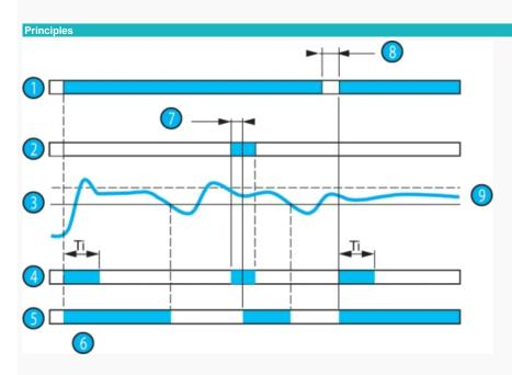
When the HSV has been configured in "memory" mode, if underspeed is detected, the output relay stays in the rest state ("alarm") irrespective of any subsequent change in the speed of the process.
