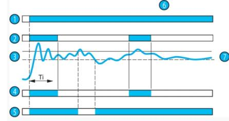
It is possible to inhibit the HSV relay by closing external contact S2 until the process has reached its nominal speed.
