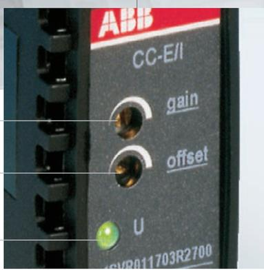
The product range CC-E for analog signal conversion includes 79 devices in four functional groups (standard signals, temperature measurement by means of PT100 sensors or by means of thermocouples types J and K, current measurement). Each functional group includes one universally configurable device as well as single-function devices. Supply voltage is 24 V DC or 110 - 240 V AC.
