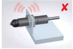
My-Com precision switch must be securely fixed into place. To ensure flawless operation, make sure the support is not subject to vibrations. Strong vibrations and high acceleration might entail switching errors caused by the inertia of the contact ball.
