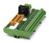
16-channel digital input module with spring-cage connection and redundant voltage supply. Suitable for Yokogawa SDV 144 card.
