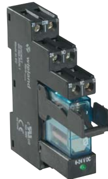
Coil voltage 24 V AC/DC Output 250 V AC / 8 A 2 Changeover contact Approvals: , in preparation
