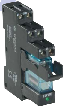
Coil voltage 12 V AC/DC Output 250 V AC / 10 A 1 Changeover contact Approvals: , in preparation
