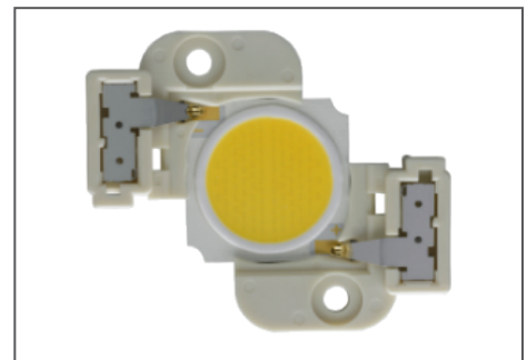
LED Array Holder for Citizen Arrays (Two-piece option shown as reference)
