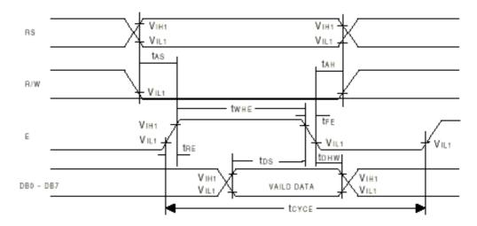
Figure 2. Bus Write Operation Sequence (Writing out data from NT7603 / NT7613 to MPU)
