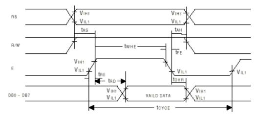
Figure 1. Bus Read Operation Sequence (Reading out data from NT7603 / NT7613 to MPU)
