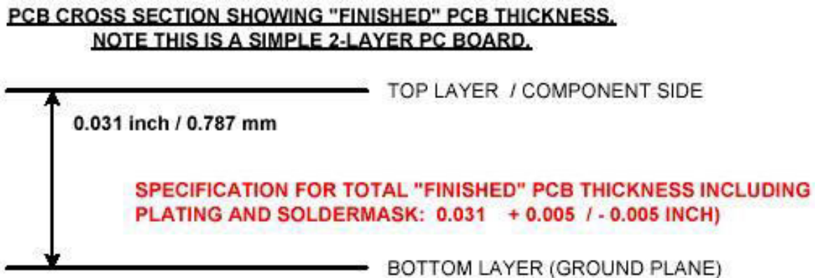
Figure 7. Cross-Section of +12 Volt Striplight PCB.
