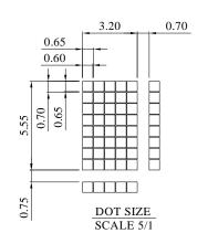
The non-specified tolerance of dimension is ; 0.3 mm.
