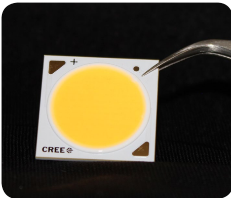
Figure 6: Correct and incorrect handling of CX family LED with fingers and tweezers
