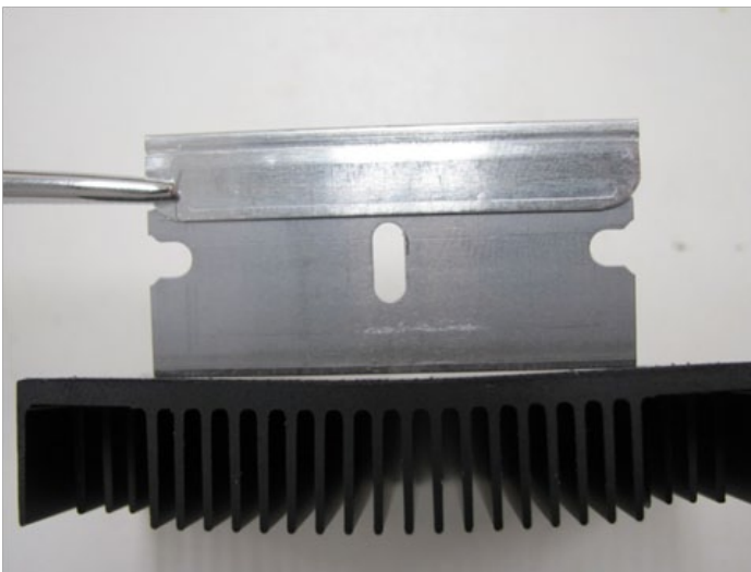
Figure 12: Checking heat sink flatness, left: a gap below the razorblade edge, right: no gap below the razorblade edge
