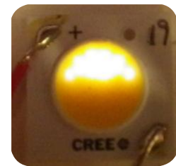
Figure 4: Partially illuminated CX family LED due to damaged bond wires
