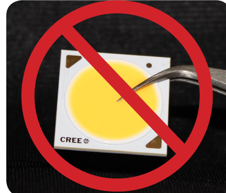
Figure 6: Correct and incorrect handling of CX family LED with fingers and tweezers
