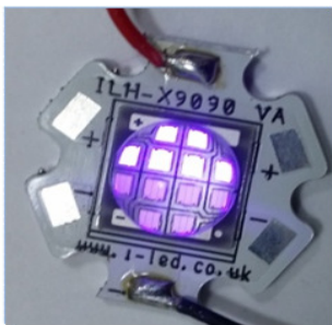
The emitter situation with 1mA driving
