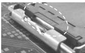
Fig 1-1 "Flat" tab cap Fig 1-2 "Raised" tab cap There are 2 type PnP cap exists, but the usage is same
