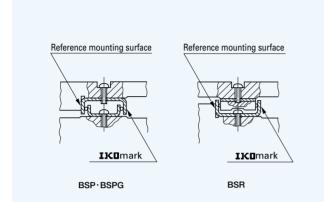
Fig. 1 Reference mounting surface
