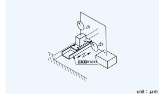
Parallelism in opera-Parallelism in operation Stroke length between slide unit center tion between slide unit mm center and mounting and reference mounting surface of track rail surface of track rail ⊿1 ⊿2 incl. over 18 3 6 — 30 4 8 18 30 50 5 10 80 6 12 50
