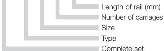
This order example (TK-01-15-2, 500) corresponds to a complete DryLin® system of size 15 with 2 carriages and 500 mm rail length.
