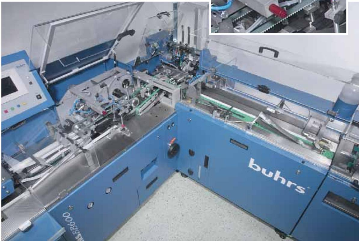
DryLin® T linear guide systems are used in these enveloping machines to guide a suction opener for envelopes. The guide system must have low clearance, be maintenance-free and not require any lubrication.
