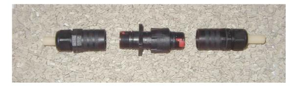
2 samples are placed for 250 hours in a dry heat chamber ( $125^{\circ}$ ). 1 sample without aging is used a reference.
