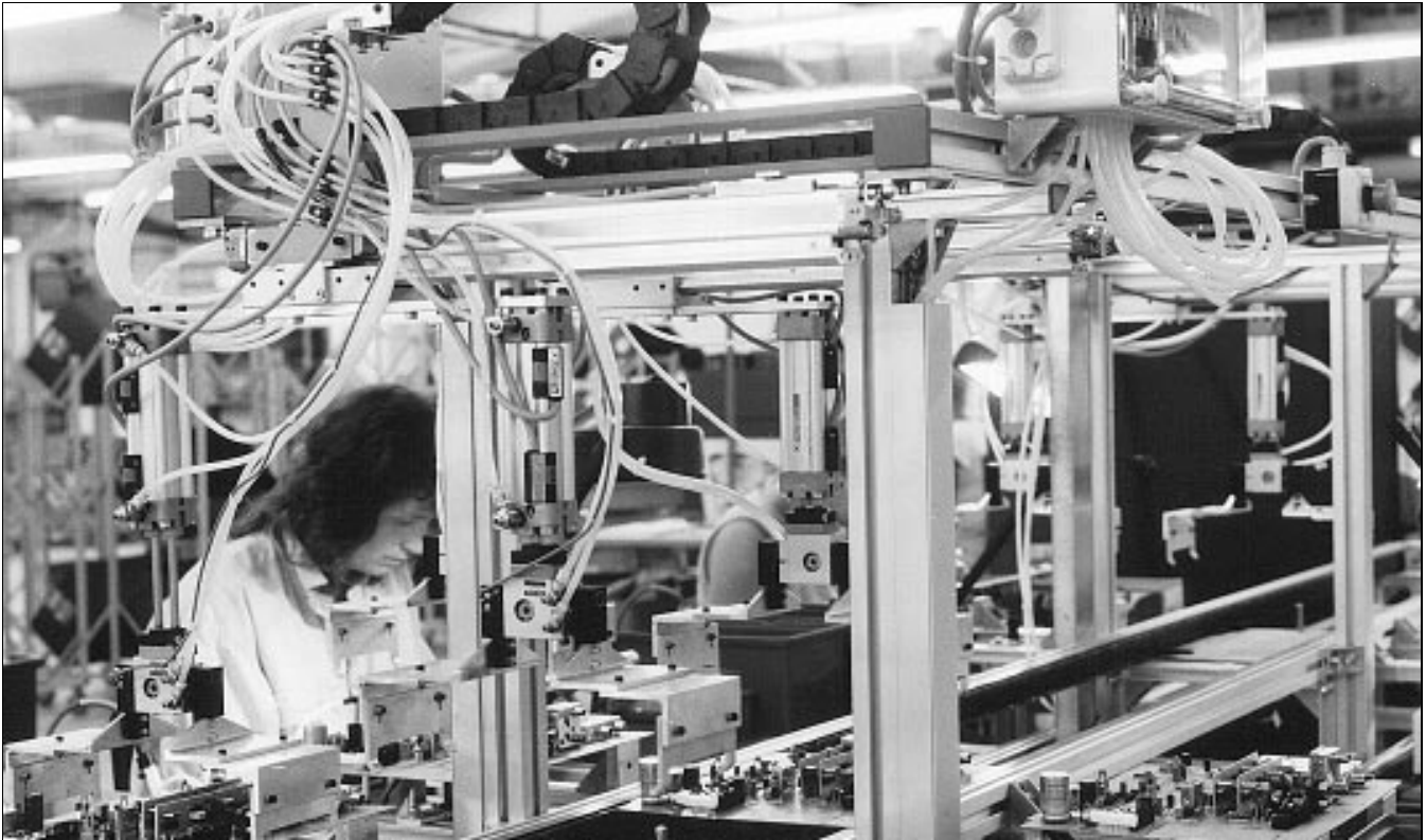
FlexLink structural system XC Close-up view of a handling unit on an assembly and test line for circuit boards.
