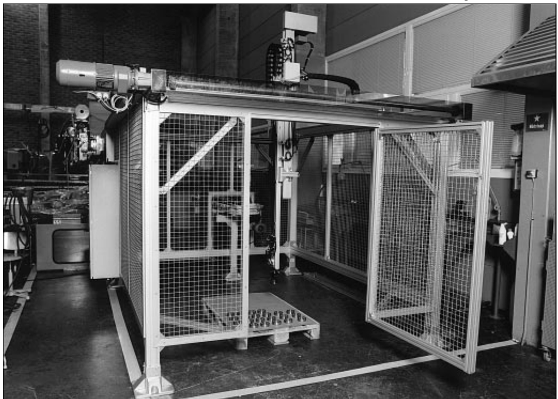
FlexLink structural system XC Automatic palletizer for bearings, feed-out side. Built with linear drive units XRH/XRL. Training site.
