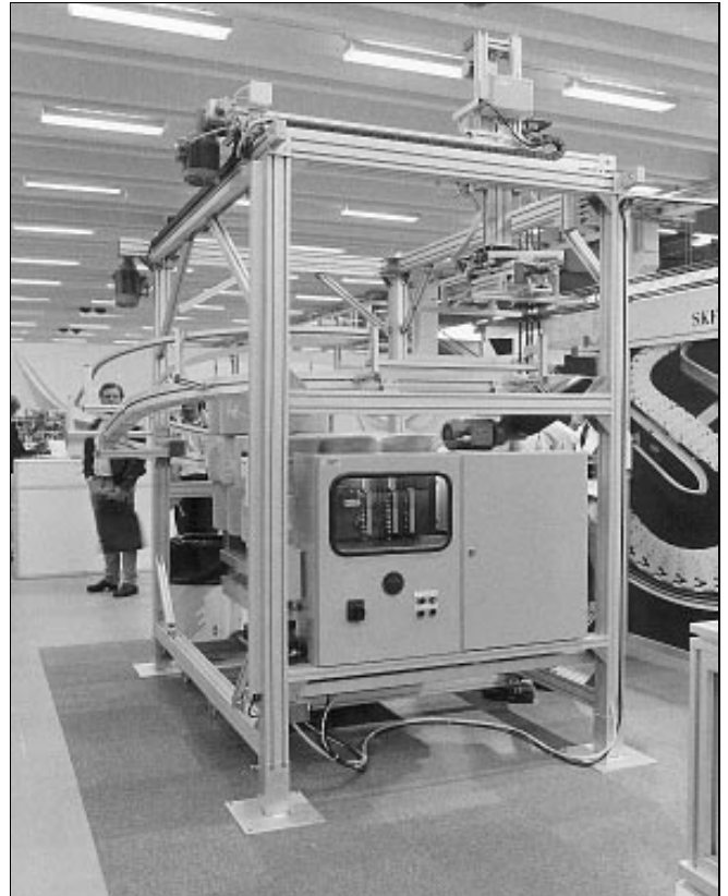
FlexLink structural system XC Automatic palletizer for industrial paper rolls.
