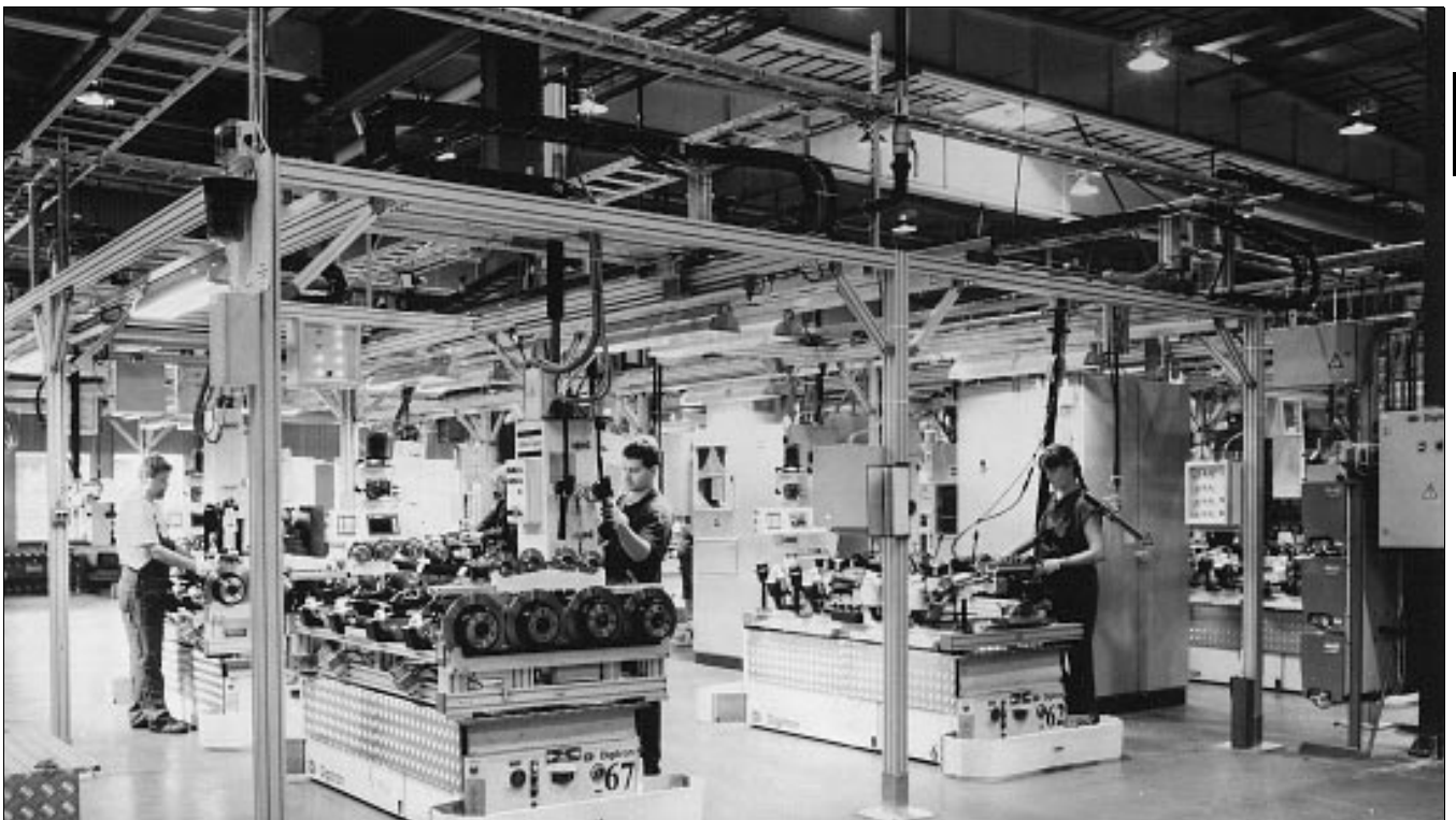
FlexLink structural system XC XC gantry framework with integrated linear motion and fixtures in an assembly cell for motor vehicle parts.
