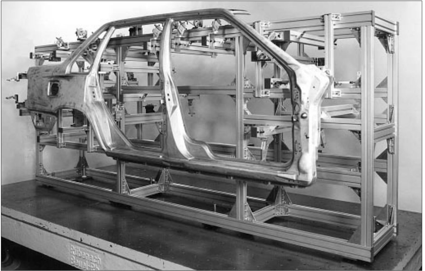
FlexLink structural system XC Tailor-made rigging system for inspection of welded car chassis assemblies.
