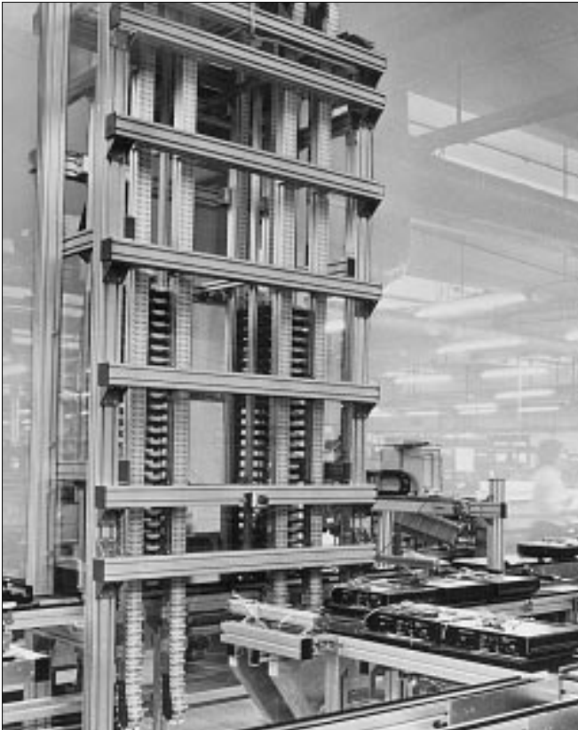
FlexLink structural system XC Twin-tower pallet store in an assembly line for satellite receivers.
