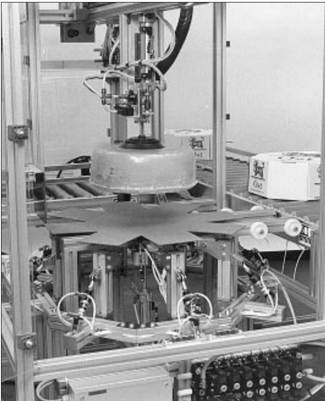
FlexLink structural system XC Close-up view of pick-and-place unit for cheese.
