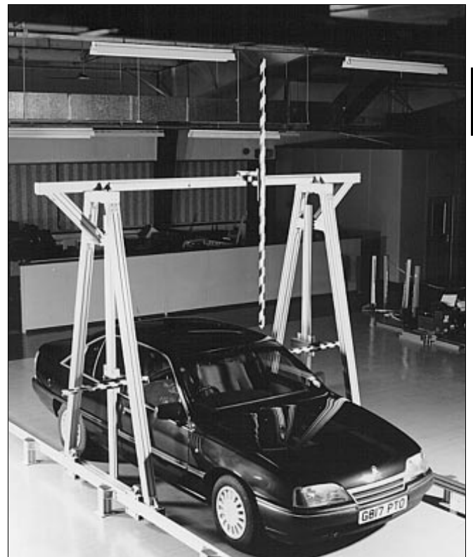
FlexLink structural system XC Three-axis crash test measuring gantry for cars.
