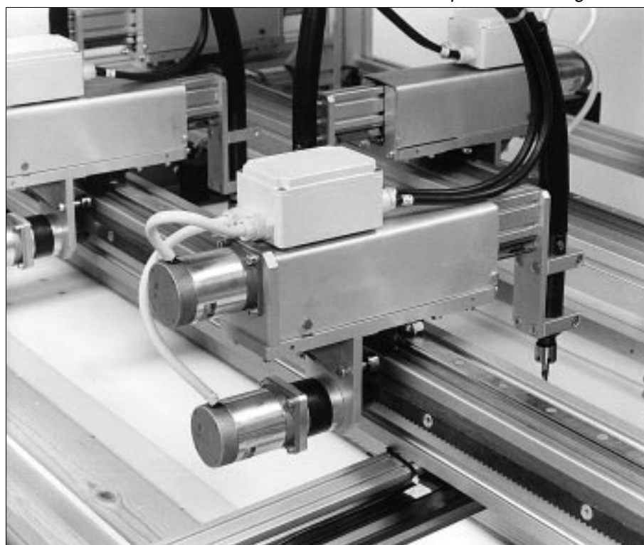
FlexLink structural system XC Close-up view of drilling unit.
