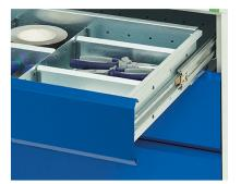
Standard fitment drawers are 50Kg U.D.L. capacity with 100% extension, roller bearing slides, for ease of action even under full load.
