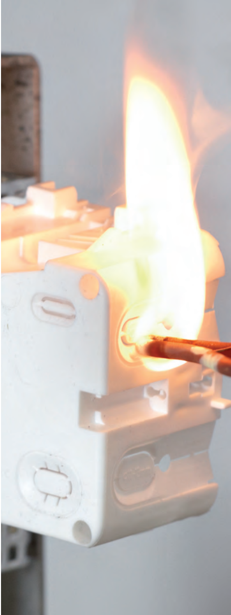
Glow-wire testing VDE
