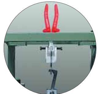
Testing adherence of the PVC coatings
