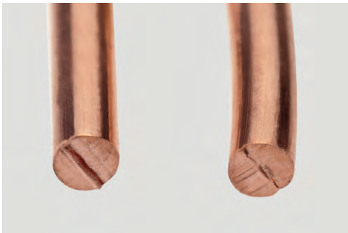
Cut with 79 42 125 (without bevel)
