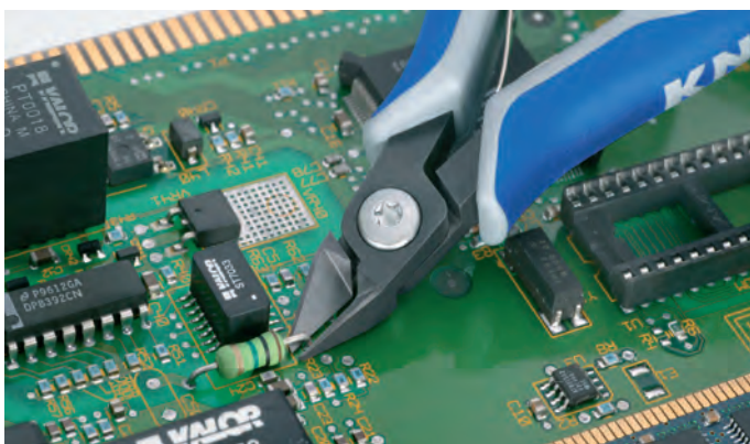
Cut with 79 42 125 (without bevel)
