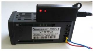
Figure 3: Inserting Programming module on UR4848xx
