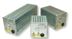
Pentagon Anti – Condensation heaters have been designed for use in switch and control gear cubicles, where a low wattage heater is required to prevent condensation. They comprise a Pentagon vitreous enamelled resistor mounted in a sheet steel case and having a removable perforated sheet steel cover. There is a cable entry grommet at each end and M4 terminal screws are provided on the resistor. Cable connection is via the M4 screws or 6.3mm push on receptacles
