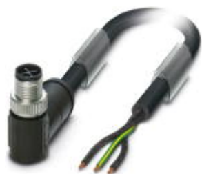
Power cable, 3-position, PVC, black, Plug angled M12 SPEEDCON, S-coded, on free cable end, Cable length: 1 m, For AC current up to 16 A/230 V
