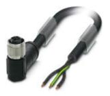
Power cable, 3-position, PVC, black, free cable end, on Socket angled M12 SPEEDCON, S-coded, Cable length: 1 m, For AC current up to 16 A/230 V
