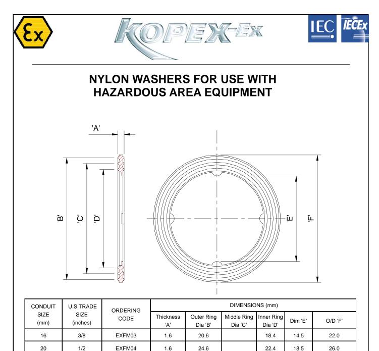
Washers EXFM03, EXFM04 AND EXFM06 only have two seal protrusions
