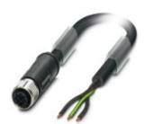
Power cable, 3-position, PVC, black, free cable end, on Socket straight M12 SPEEDCON, S-coded, Cable length: 10 m, For AC current up to 16 A/230  $\rm V$
