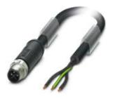
Power cable, 3-position, PVC, black, Plug straight M12 SPEEDCON, S-coded, on free cable end, Cable length: 10 m, For AC current up to 16 A/230 V
