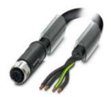
Power cable, 4-position, PUR halogen-free, black-gray RAL 7021, free cable end, on Socket straight, S-coded, Cable length: 10 m, For AC current up to 12 A/630 V
