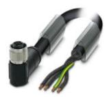
Power cable, 4-position, PUR halogen-free, black-gray RAL 7021, free cable end, on Socket angled M12 SPEEDCON, S-coded, Cable length: 5 m, For AC current up to 12 A/630 V
