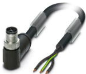
Power cable, 3-position, PVC, black, Plug angled M12 SPEEDCON, S-coded, on free cable end, Cable length: 5 m, For AC current up to 16 A/230 V
