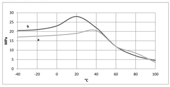
Roller peel test (ISO 4578)(typical average values) - Cure : 16 hours/40°C 5 N/mm
