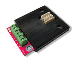
The DCP temperature controller provides closed loop, temperature sensitive speed control for ebm-papst 4-wire PWM controlled DC fans. The controller voltage is matched to the fan so that with its very low power consumption, there is no need for a separate, dedicated power supply.
