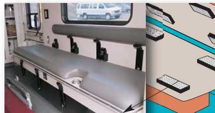
With 3M™ Dual Lock™ Reclosable Fasteners, the wall panels, cushions, and other components inside an emergency vehicle are easily removed without tools for cleaning and disinfecting.
