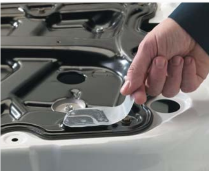
303 3M™ UHMW-PE Tape 5425 provides a “slip plane” effect between incompatible surfaces to help reduce squeaks and rattles.
