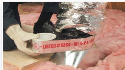
317 To seal fiberglass duct board and flexible duct systems, Scotch® Foil Tape 3326 meets the performance requirements for UL 181A-P and UL 181B-FX.
