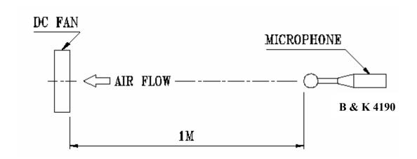
Noise is measured under Rated Voltage in free air in the anechoic chamber with B & K Nexus 4350 conditioning amplifier, with B & K 4190 microphone at a distance of one meter from the fan intake. The background noise is 18dBA max under the ISO-3745 Standard.
