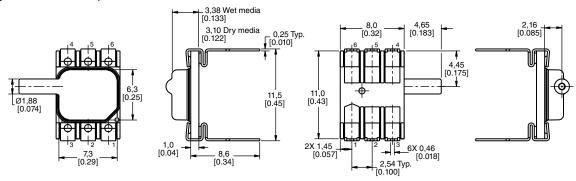
Figure 2. DIP Package Dimensional Drawings (continued)
