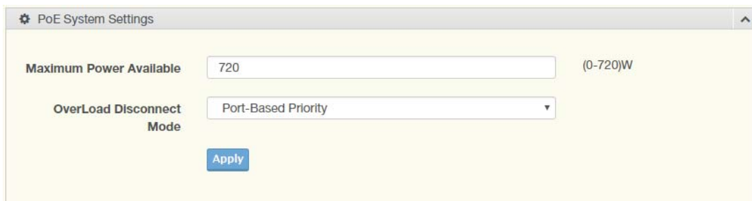
Figure 110: Management > Power Over Ethernet > PoE System Settings
