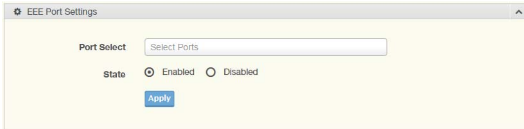
Figure 59: L2 Switching > 802.3az EEE
