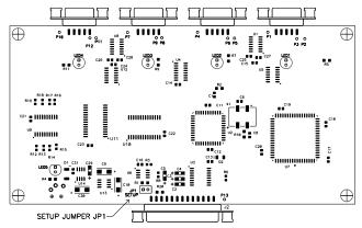
Figure 4.1 Setup Jumper Location
