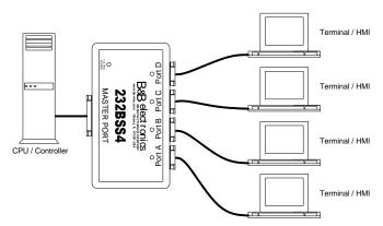
Figure 2.1. Multiple Terminals to a Host Controller
