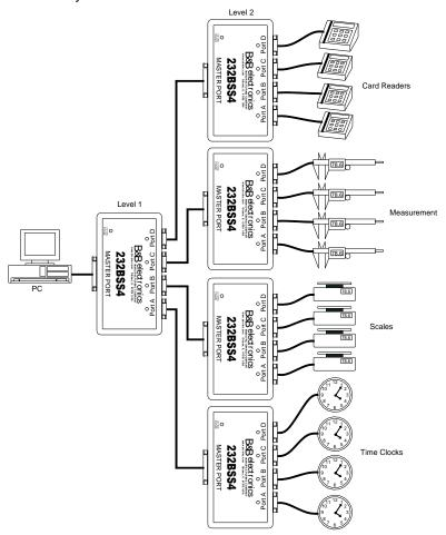
Figure 2.3. Expanding the Number of Slave Ports
