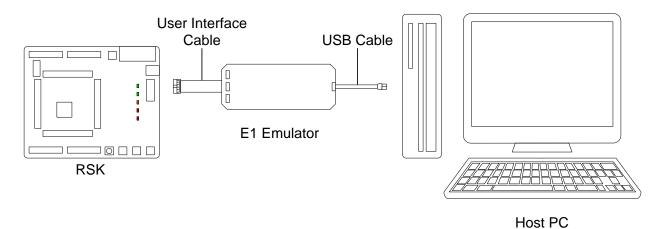
Figure 4-2: Debugger Connection Diagram
