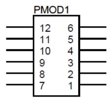
Figure 5-1: Digilent Pmod™ Compatible Header Pin Numbering
