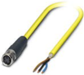
Sensor/actuator cable, 3-position, PVC, yellow, shielded, free cable end, on Socket straight M8, cable length: 5 m
